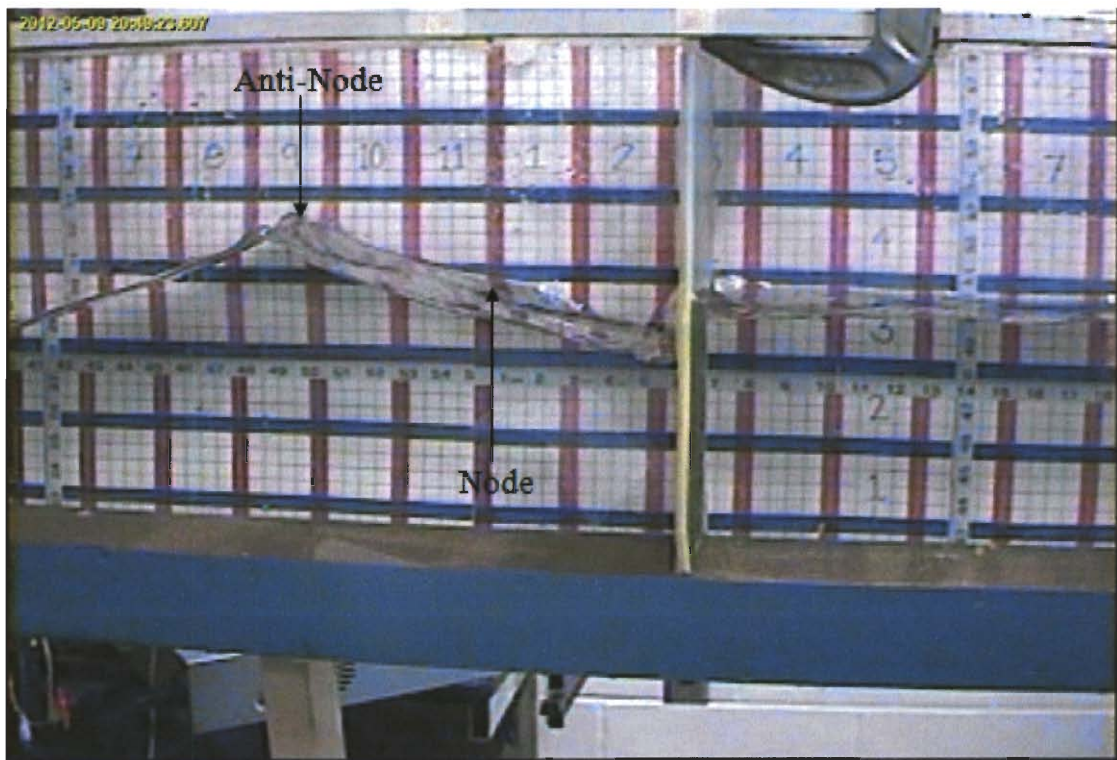
Figure 4.12 Node and anti- node locations for steepness comparison. It is seen the wave is steeper on either side of the anti-node than at the node.
